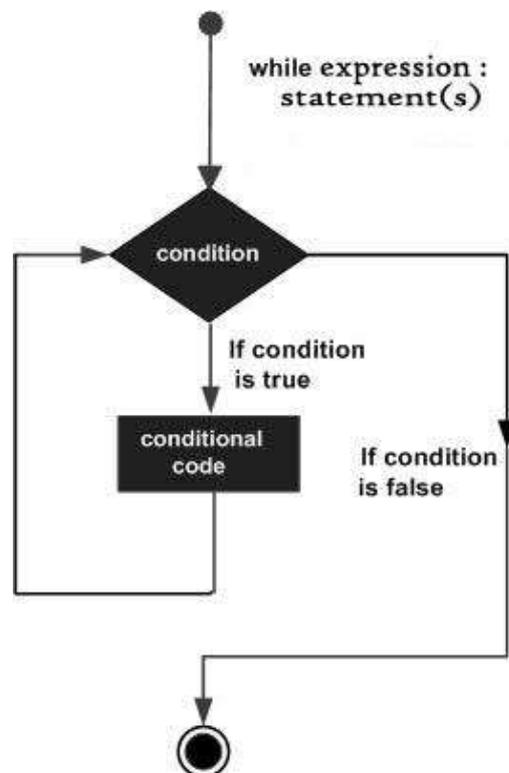
Here, key point of the *while* loop is that the loop might not ever run. When the condition is tested and the result is false, the loop body will be skipped and the first statement after the while loop will be executed.
